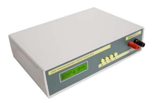
The 2090 provides the solution to the requirement of a programmable resistance box in one compact unit. Connect the 2090 to the serial COM port of a P.C. and automate almost any task performed by a standard resistance box saving time and reducing errors.
